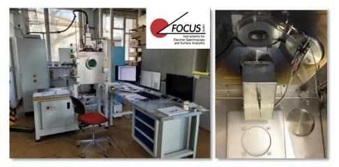
Unique wire-fed micro e-beam AM setup Combining 3D Printing Techniques and Electron Microscopy
