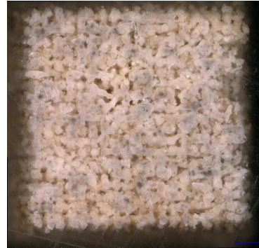
Porosity induced by hatch distance, \text{MnO}_2 dopant
