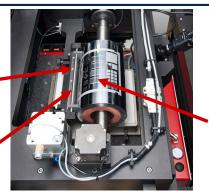
Software controlled inking via slot die head
