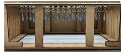
Test rig modelling pressure with distributed weights; pictured: 150g
