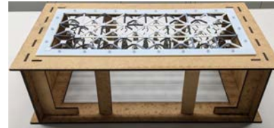
Test rig modelling pressure with distributed weights; pictured: 150g
